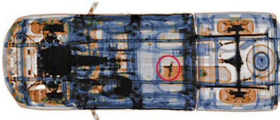
Figure 3: Transmission image from Rapiscan's Carview system. Shows how transmission X-ray scans can be used to detect hidden objects, in this case firearms.
